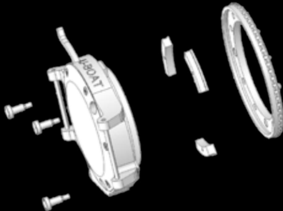
3. Remove the bezel: this also releases the three semicircular tenon joints.
