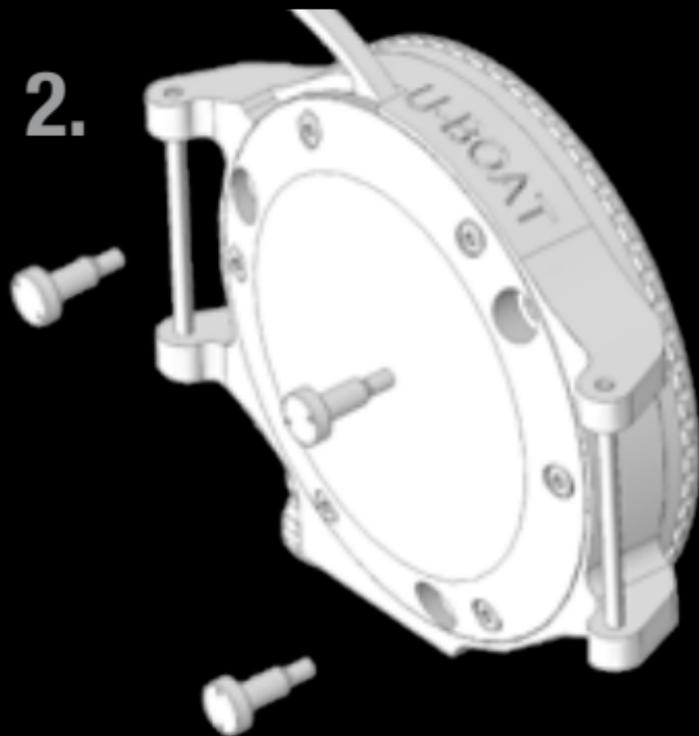
To carry out cleaning and maintenance operations on the rotating bezel, please proceed with the following dismantling steps:
