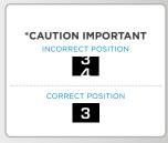
To avoid misalignment or breakage of the date click wheel when setting the date, make sure that:
