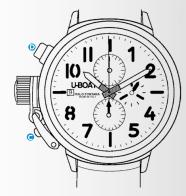
Press the (on/off) pusher  $\odot$  to start the chronograph hand and the hours/minutes totalizer.
